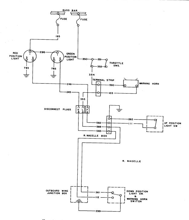
Warning Horn and Position Light Circuit
