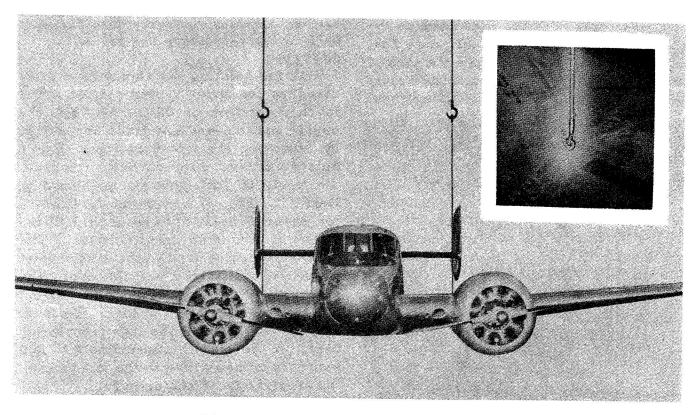
Fig. 5 Hoisting Using Two Hoists
