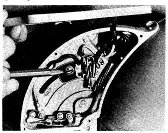
Fig. 84 Landing Light Adjustment
