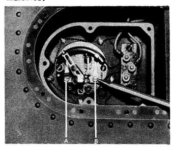
Fig. 82 Fuel Transmitter Unit Adjustment
