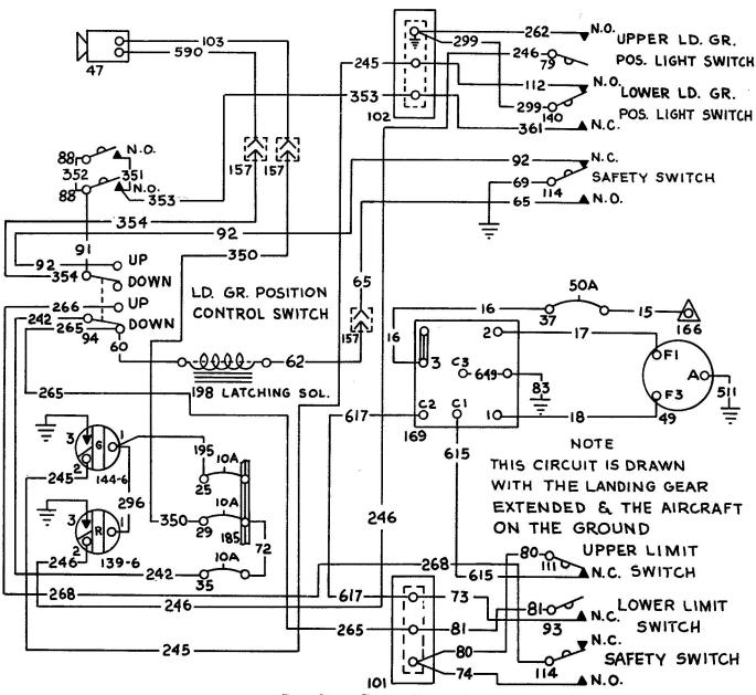
Landing Gear Circuit Aircraft Serials A-537 and After
