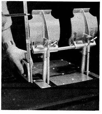
Fig. 49 Toe Brake Pedal Adjustment
