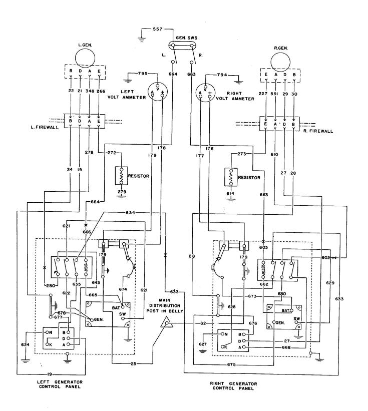
D18S Generator Circuit with Voltage Regulator on Bulkhead 5
