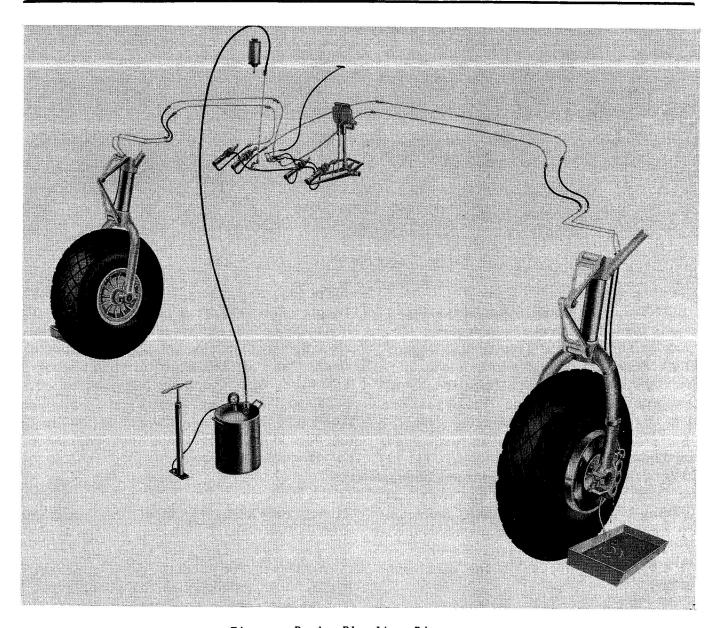
Fig. 52 Brake Bleeding Diagram
