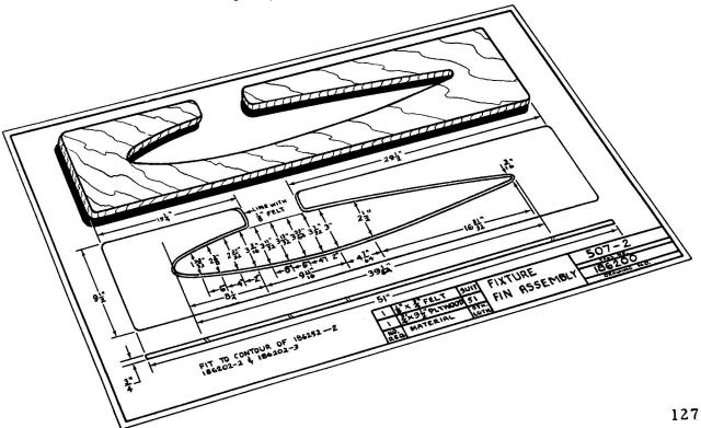
Fig. 88 Rudder Aligning Jig
