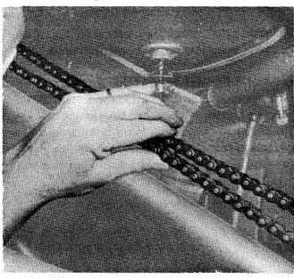
Fig. 33 Landing Gear Chain Tension
