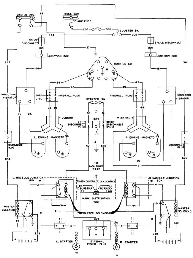
Ignition and Battery Circuit with Booster Switch
