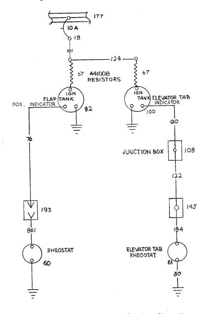
Elevator Tab and Flap Position Indicator Circuits Aircraft Serials A-402 and After
