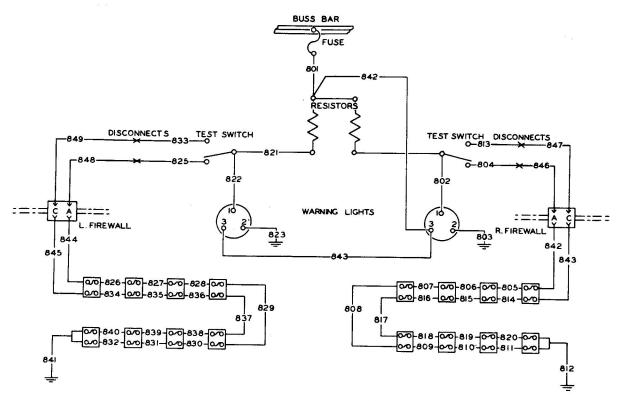
D18CT Fire Detector Circuit
