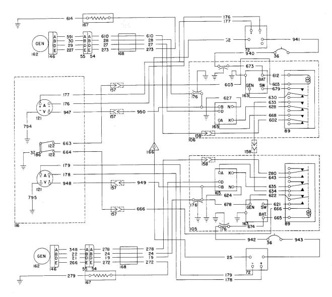
Generator Circuit with Voltage Regulator in Wing Stub Aircraft Serials A-351 and After (D-18S), A-26 and After (D18C and D18CT)
