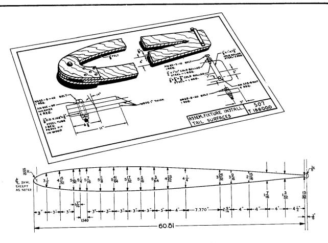
Fig. 87 Elevator, Contour, Jig
