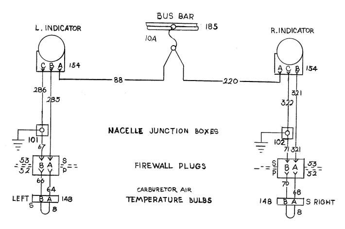
Carburetor Air Temperature Circuit Aircraft Serials A-402 to A-537
