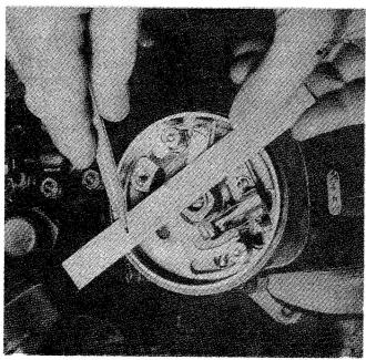
Fig. 22 Magneto Breaker Point Adjustment (Scintilla)
