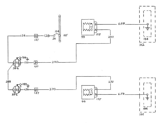
Vacuum Light Circuit Aircraft Serial A-537 and After
