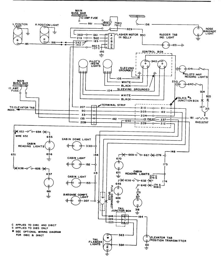
Navigation, Instrument, and Interior Lighting Circuit
