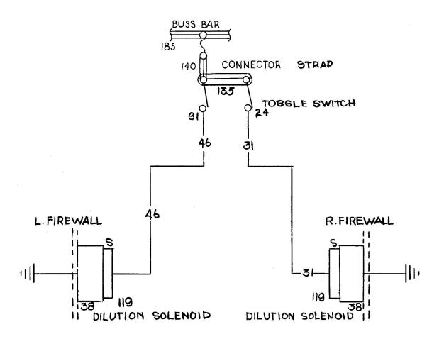
Oil Dilution System Aircraft Serials A-402 to A-537
