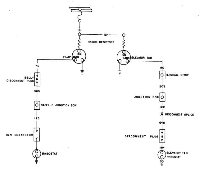
Elevator, Tab and Flap Position Indicator, Circuits.
