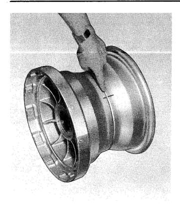
Fig. 38 Main Wheel Balance Mark WHEELS
