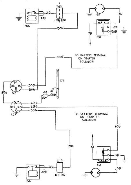
Propeller Feathering Circuit Aircraft Serials A-402 and After
