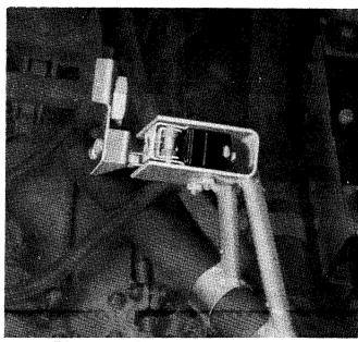
Fig. 35 Upper Limit Switch Adjustment
