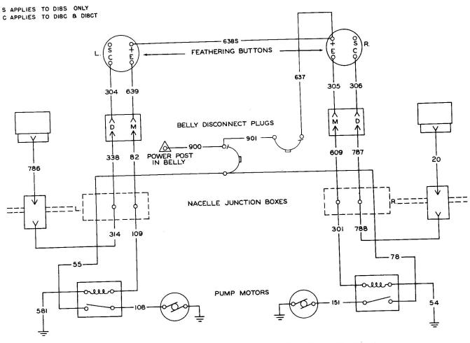
Propeller Feathering Circuit with Two Circuit Breakers
