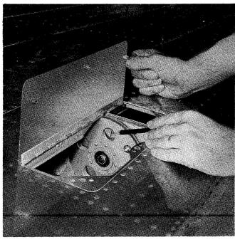
Fig. 60 Aileron Travel Stop Adjustment.
