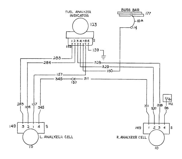
Fuel Analyzer Circuit Aircraft Serials A-402 and After
