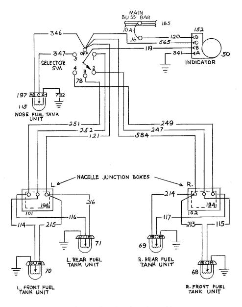
Fuel Level Indicator Circuit Aircraft Serials A-402 and After
