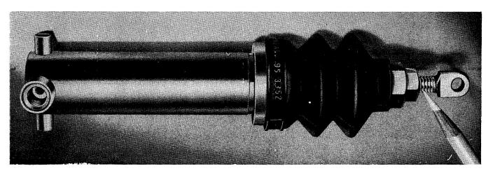
Fig. 53 Master Cylinder Clevis Adjustment
