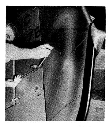
Fig. 70 Rudder Position Setting
