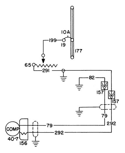
Compass Light Circuit Aircraft Serials A-537 and After
