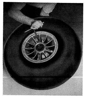
Fig. 41 Removing Locking Nuts
