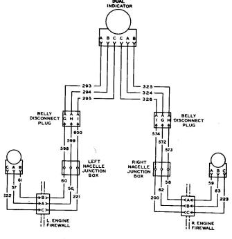
D18C Tachometer Circuit
