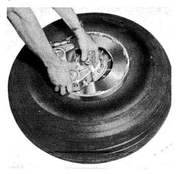
Fig. 39 Brake and Axle Assembly in Wheel
