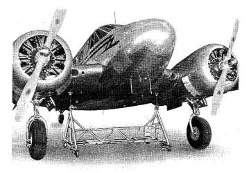
Fig. 3 Main Wheel Jacking
