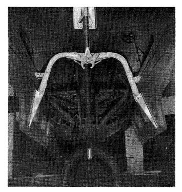
Fig. 55 D18C Landing Gear Door Linkage
