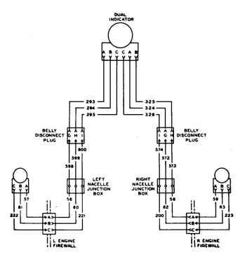
D18S Tachometer Circuit
