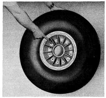
Fig. 43 Assembling Tire and Tube to
