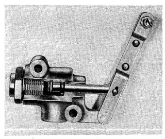
Fig. 51 Cutaway View of Parking Brake
