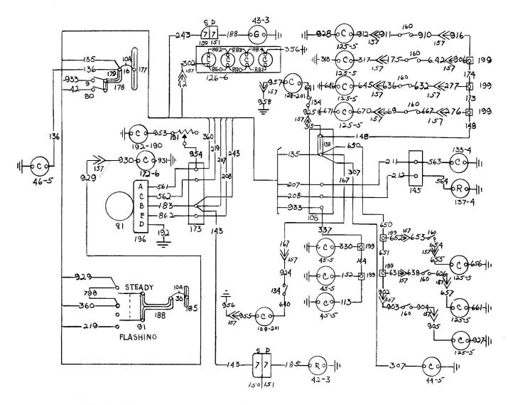
Navigation, Instrument, and Interior Lighting Circuits Aircraft Serials A-537 and After
