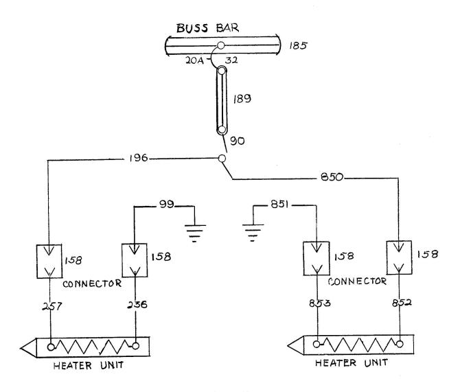
Pitot Heat Circuit Aircraft Serials A-537 and After
