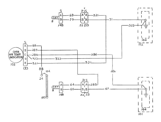
Carburetor Air Temperature Circuit Aircraft Serials A-537 and After
