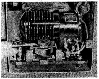
Fig. 81 Voltage Regulator Adjustment
