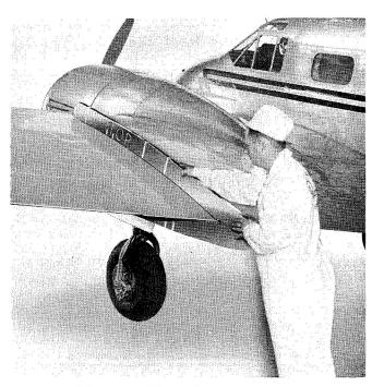
Fig. 79 Flap Contour Jig
