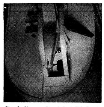
Fig. 63 Elevator Travel Stop Adjustment
