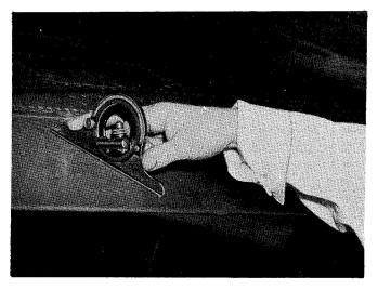
Fig. 59 Aileron Position Setting
