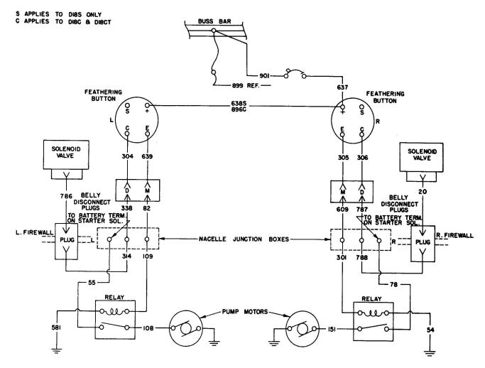
Propeller Feathering Circuit with One Circuit Breaker.
