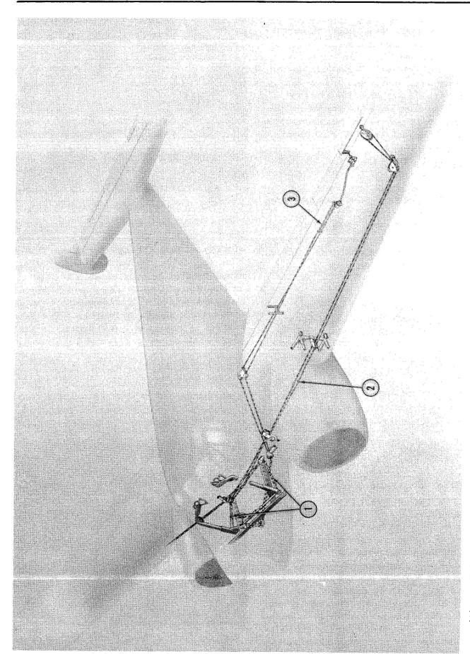
3. Aileron Tab Cable Turnbuckles 1. Aileron Balance Cable Turnbuckles 2. Main Aileron Cable Turnbuckles
