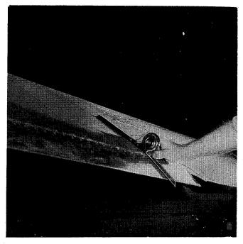
Fig. 67 Elevator Tab Position Setting
