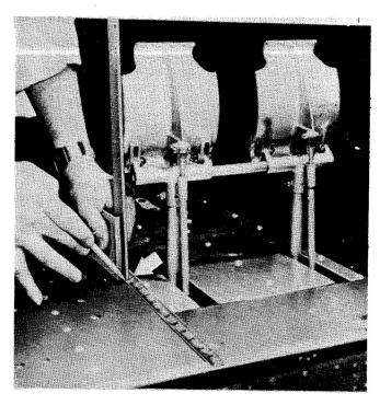
Fig. 74 Rudder Pedal Setting
