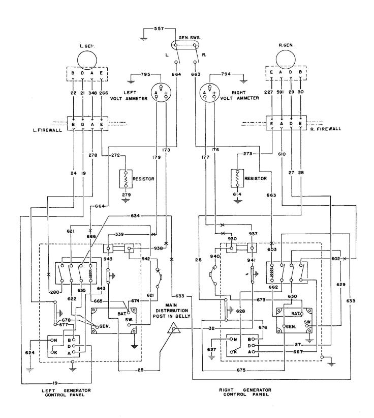
D18S Generator Circuit with Voltage Regulator in Wing Stub
