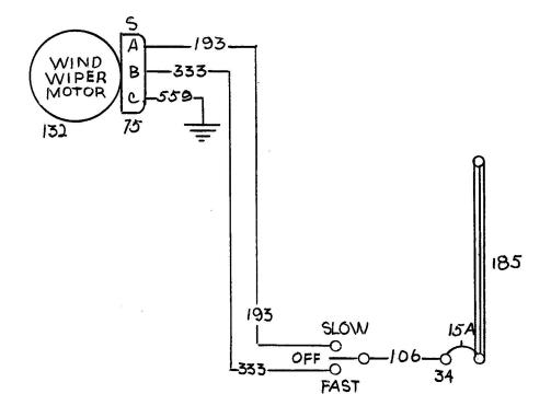
Windshield Wiper Circuit Aircraft Serials A-537 and After
