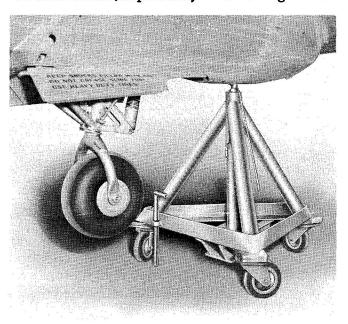
Fig. 4 Tail Wheel Jacking
