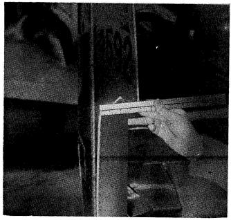
Fig. 75 Rudder Tab Position
