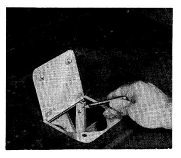
Fig. 71 Rudder Travel Adjustment
