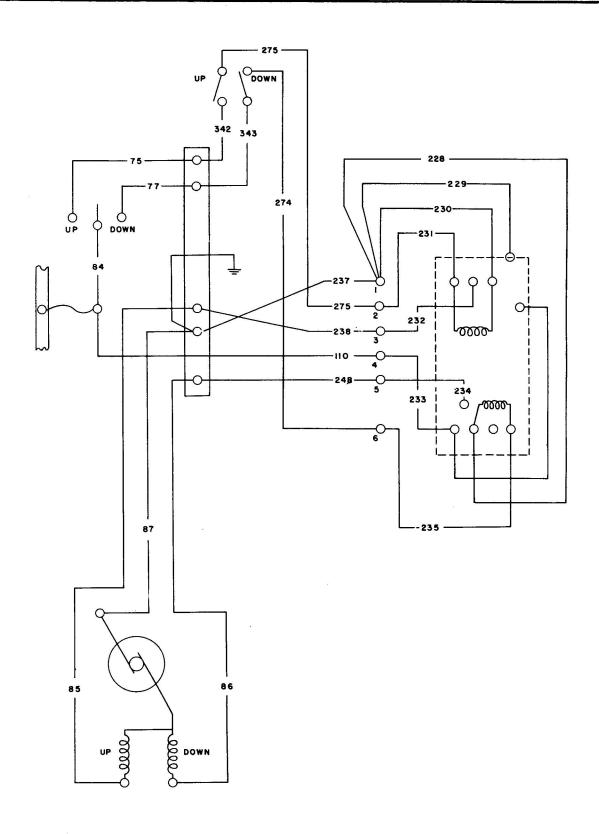
Flap Circuit with General Electric Dynamic Brake Relay
