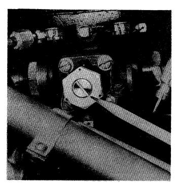
Fig. 18 Fuel Pressure Adjustment
