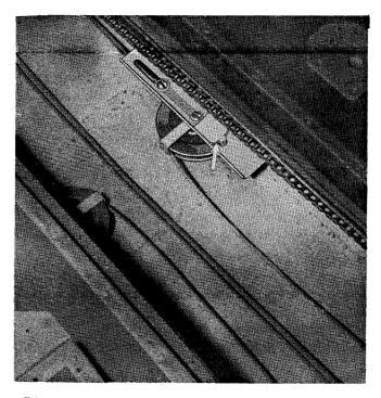
Fig. 73 Rudder Reduction Rigging Blocks
