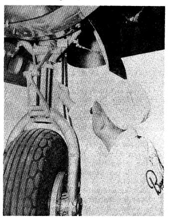
Fig. 36 Safety Switch Adjustment
