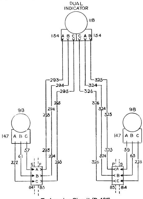
Tachometer Circuit (D-18S) Aircraft Serials A-402 and After
