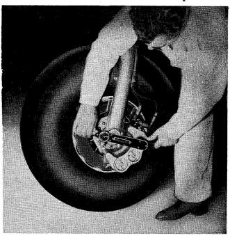
Fig. 46 Brake Packing Nut Torque
