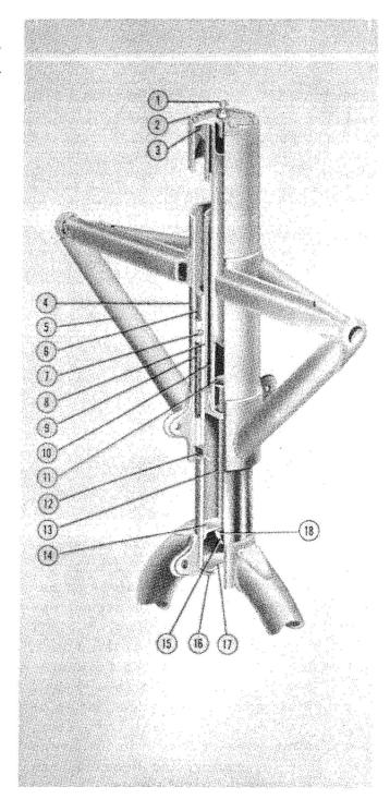
Fig. 37 Main Landing Gear Shock Absorber
