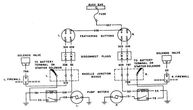
Propeller Feathering Circuit with Fuse
