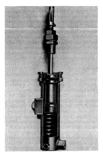
Fig. 47 Cutaway View of Master Cylinders
