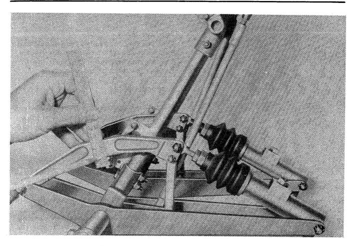
Fig. 48 Master, Cylinder, Linkage Adjustment
