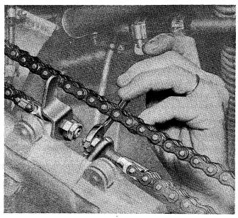
Fig. 32 Landing Gear Chain Adjustment
