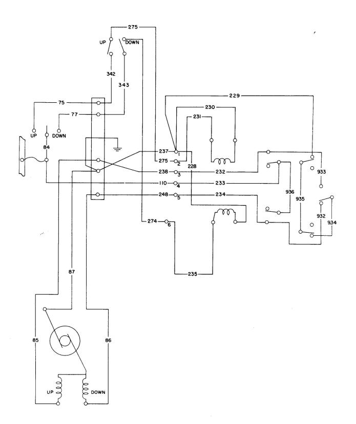
Flap Circuit with Phillips Dynamic Brake Relay
