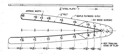
Fig. 89 Flap Contour Jig
