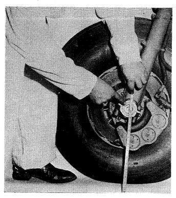
Fig. 11 Main Wheel Tire Inflation be inflated so the centerline of the axle is 6 inches above the ground (See Fig. 12).
