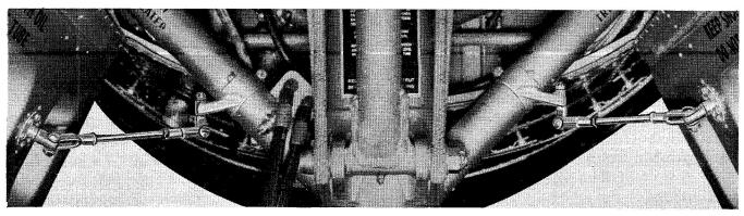
Fig. 54 D18S Landing Gear, Door, Linkage
