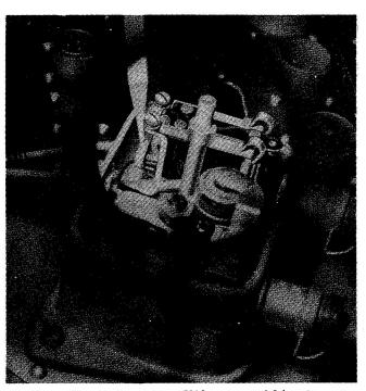
Fig. 80 Induction Vibrator Adjustment
