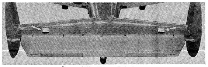
Fig. 72 Rudder Balance Cable Location
