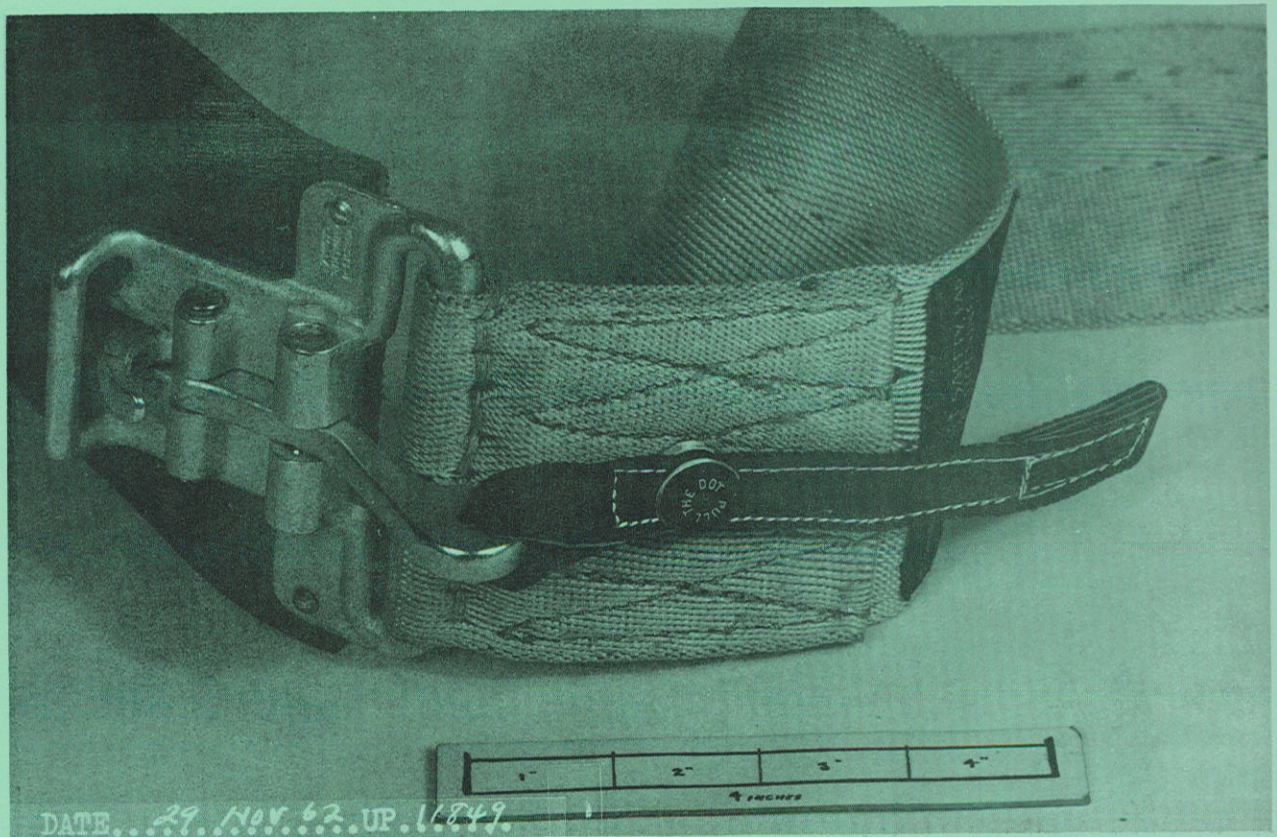
Figure 3 Lap Belt Tab Installation as Fitted to C2 Ejection Seat
