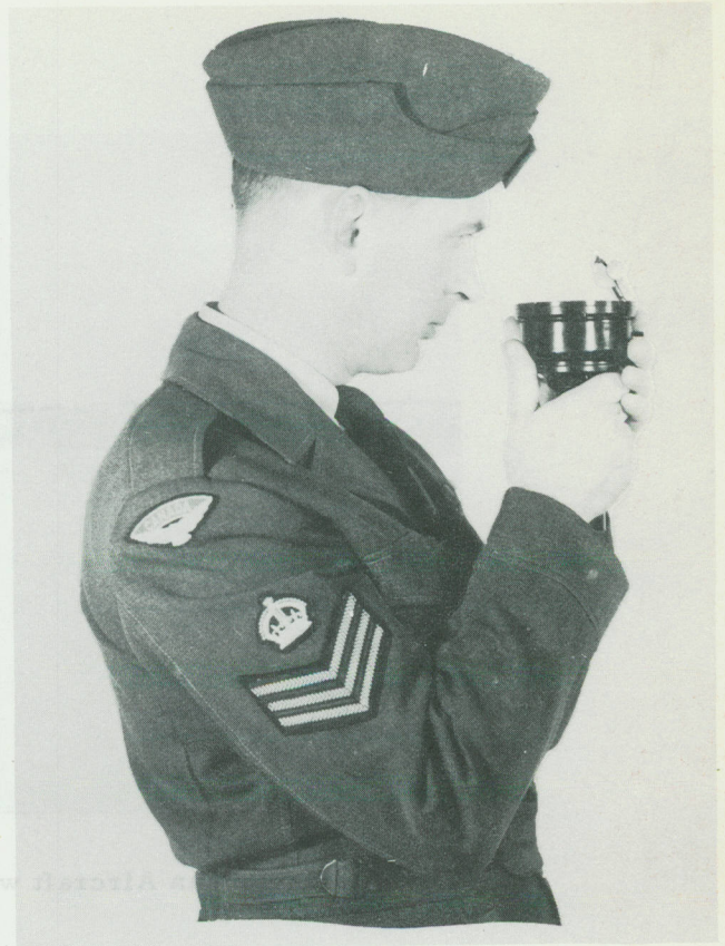
Figure 5-4 Side View of Correct Method of Holding the Sighting Compass
