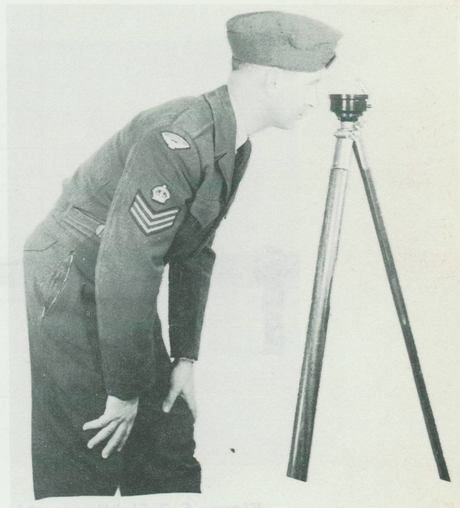
Figure 5-5 Side View - Observer Using Sighting Compass Fitted to Tripod
