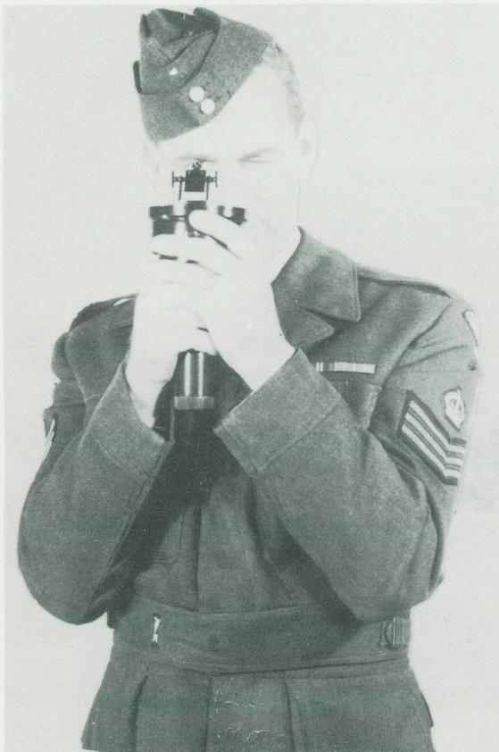
Figure 5-3 Front View of Correct Method of Holding the Sighting Compass
