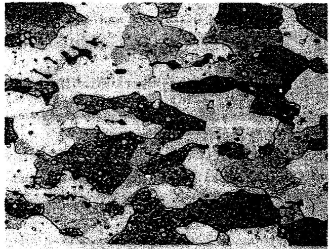
Figure 8-10 Insufficient Temperature Heat Treat R301 Alloy
