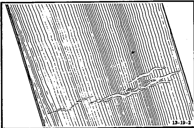
Figure 19-5 Compression Failure in Sitka Spruce
