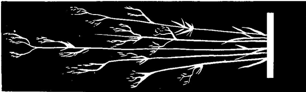
Figure 6 Sparks From Malleable Iron
